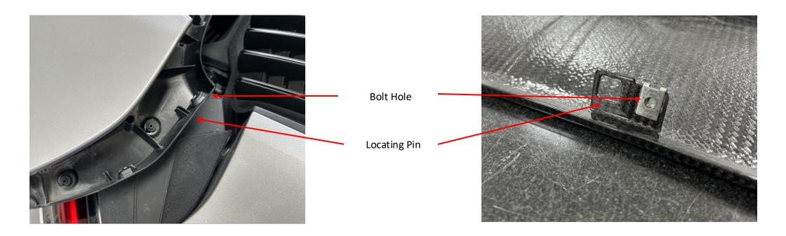
• The ducktail spoiler can now be added to the car. In the lower standard spoiler moulding you can see a male locating pin and a bolt hole at each of the 8 attachment points. The pin should be aligned with the square hole in the mounting tab and the bolt hole with the with the metal clip added to the mounting tab.
